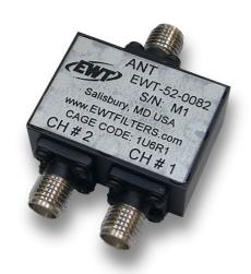
Model EWT-52-0082 is a miniature diplexer that covers the bands DC-1300 MHz and 3500-5500 MHz. The lower passband exhibits less than .50 dB insertion loss with the upper band having .75 dB max insertion loss. VSWR for both channels is less than 1.7:1. Channel to channel isolation is greater than 60 dB. The overall size is 1.05" x .75" x .45" with SMA connectors.
